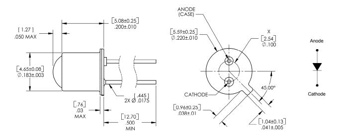
X THIS DIMENSION CONTROLLED AT HOUSING SURFACE.
