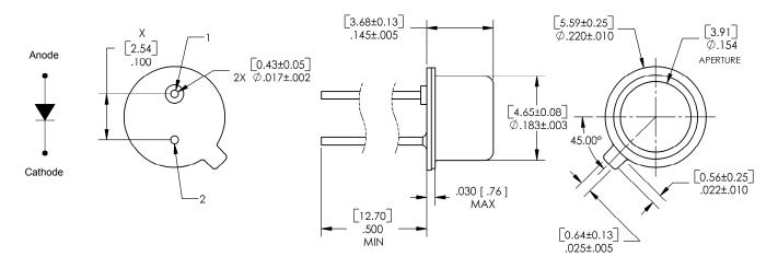
X THIS DIMENSION CONTROLLED AT HOUSING SURFACE.
